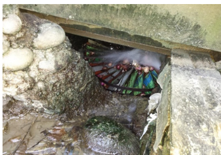
In the figure above, the turbine runs by water to rotate the upper millstone
